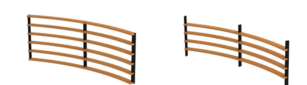
Step 3: Panel ready to be fitted, after drilling the counter-slats for the hangers (Ø 9 mm)
