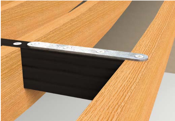
Step 2: Attach the slat using the assembly strips and 4 screws
