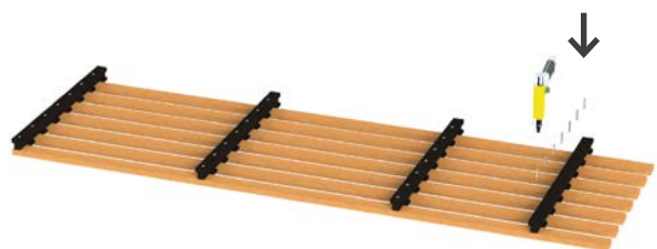
Step 4: Screw the counter-slat back on
