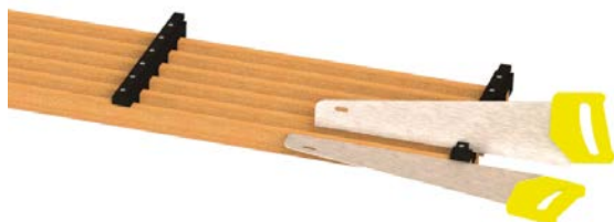
Step 5: Notch the end of the counter-slat
